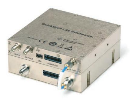
We've extended our popular QuickSyn Lite frequency synthesizers to three commonly used mmW bands—27 to 40 GHz, 50 to 67 GHz, and 76 to 82 GHz—for high-speed short-range data links, WirelessHD, IEEE 802.11ad, digital radios, automotive radars, etc. QuickSyn mmW frequency synthesizer modules are ideal for demanding application environments like field trials and embedded systems where bulky benchtop solutions have been the only choice.
