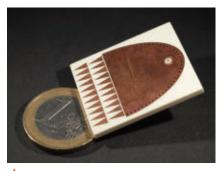
Fig. 2 Etched transition reduces the mismatch between the aperture and free space.
