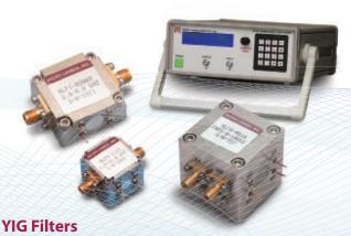
Micro Lambda Wireless offers a very extensive YIG-Tuned Filter product line with standard designs covering from 500 MHz to 50 GHz. Various package configurations utilizing from 2 stages to 8 stages in the band pass filter product lines and up to 16 stages in the band reject filter products make Micro Lambda's YIG-Tuned filter offering the largest on the market today. Miniature filters covering 1 GHz to 8 GHz, permanent magnet filters covering 4 GHz to 16 GHz, standard
