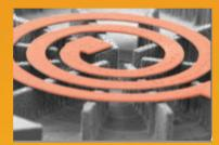
A GECCO™ High-Q Inductor. 50um wide, 5um thick, metal coil resting on 20um wide glass rails
