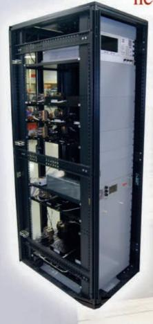
105 Fixed Filters 6 foot rack Switches Control Circuitry
