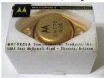
▲ Fig. 4 The 2N176 germanium transistor was rated at 6 A, 15 V, 90 W, 4 kHz, 90°C Tj max. It was the audio amplifier in a car's AM radio.
